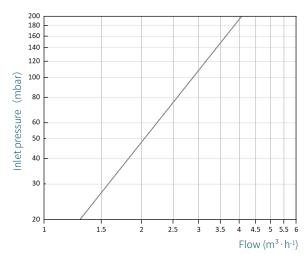
Bypass orifice diameter: 3mm.
