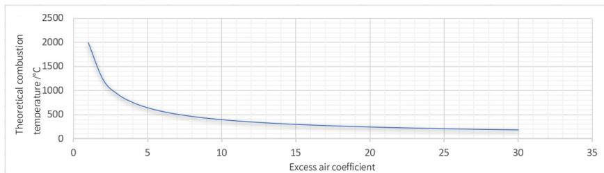
Natural gas, not preheating air, calorific value: 34500~35600 kJ·m<sup>-3</sup>.
